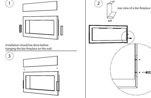
The glass must be tucked in from top to bottom.
