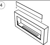
The glass should be inserted into the holders from top to bottom.
