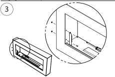
Fasten the glass holders with the help of screws and nuts included in the kit.
