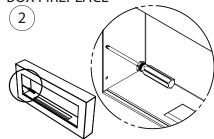
Remove mounting points with screwdriver or other tool by pressing.
